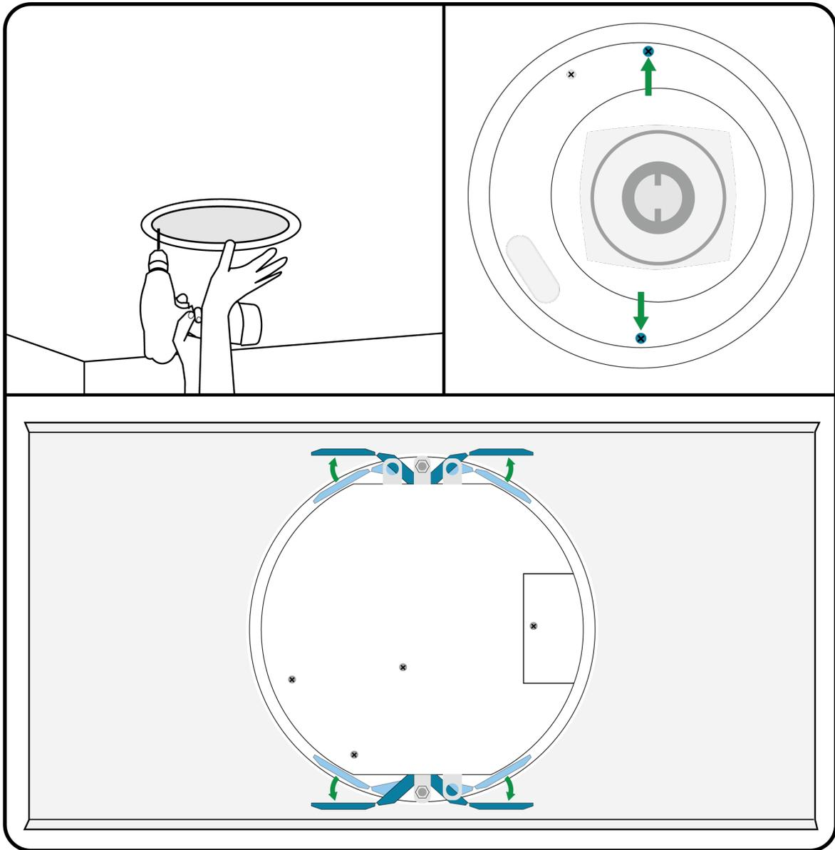
5. Slide to attach the grille safety restraint to the post on the loudspeaker. Do not unscrew the screw to attach the restraint.
