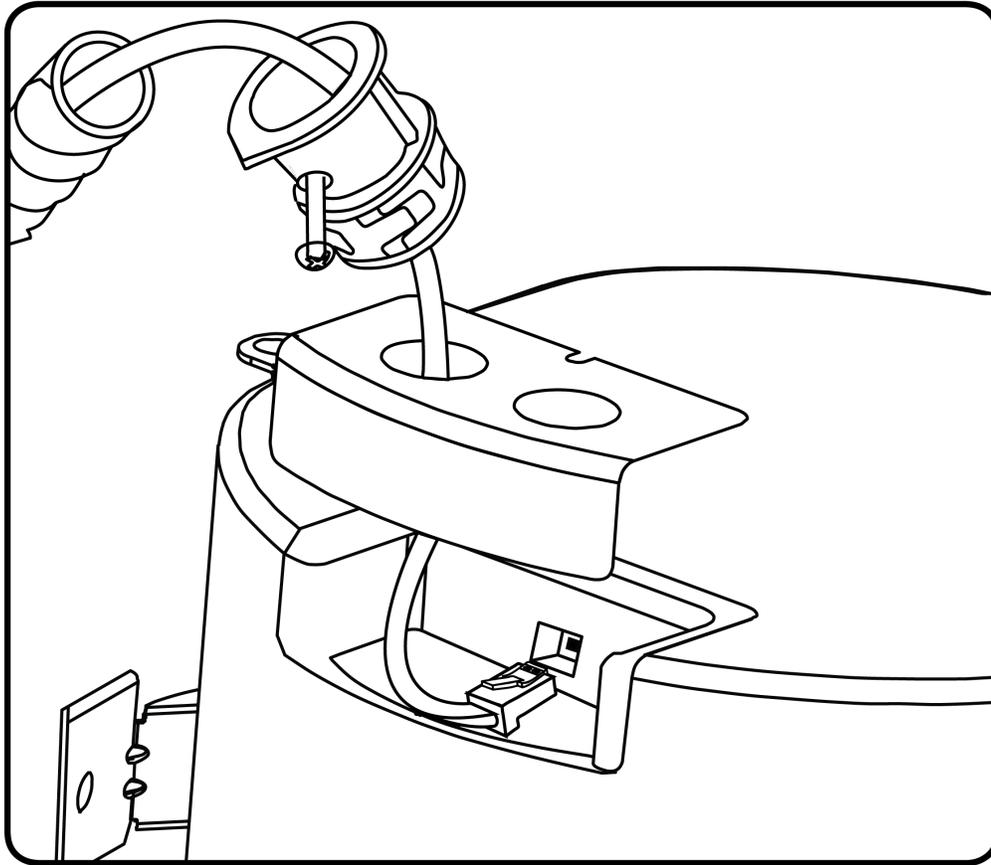
2. Attach the cover plate with the screwdriver. If using conduit, push the conduit connector into the knockout.
