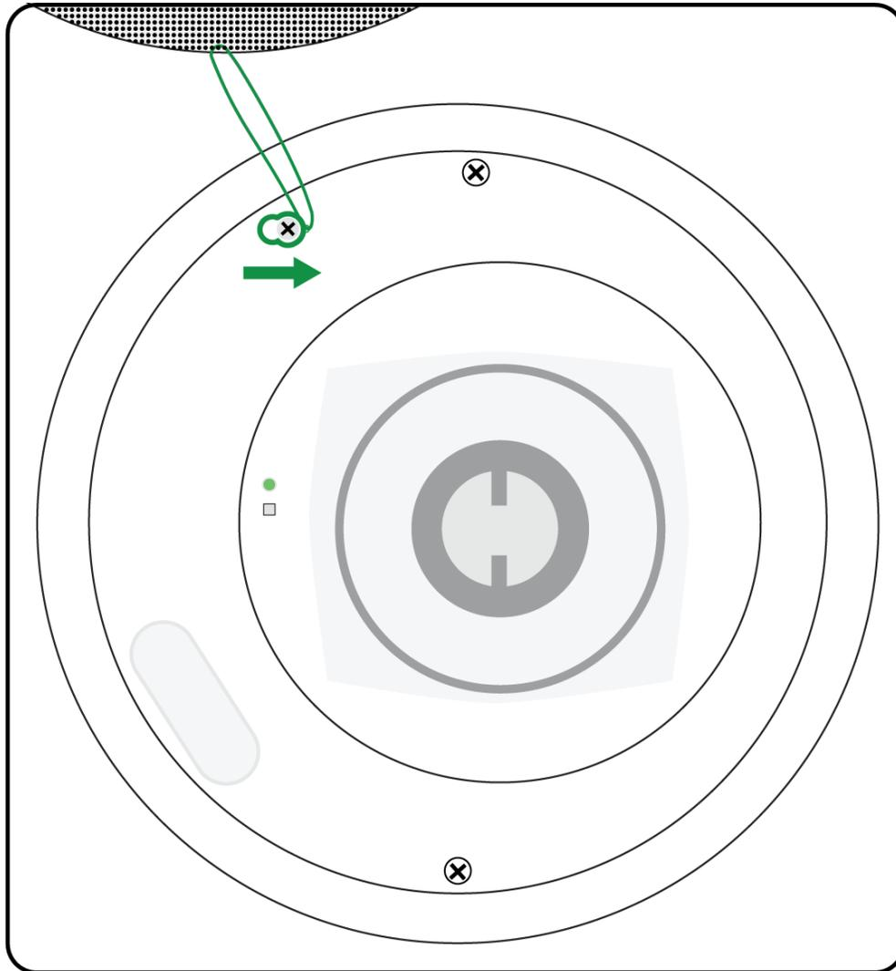
6. Attach the magnetic grille to the loudspeaker. The Shure logo is also magnetic, so you can reposition or remove it if necessary.
