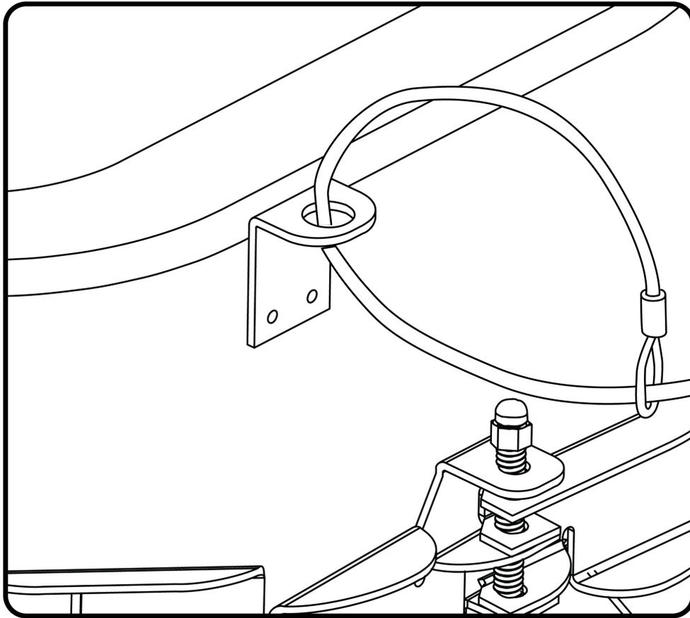
4. Place the loudspeaker in the mounting hole. Tighten the screw on each side of the loudspeaker until each mounting arm fully expands to secure the loudspeaker. Do not over-tighten the screws.
